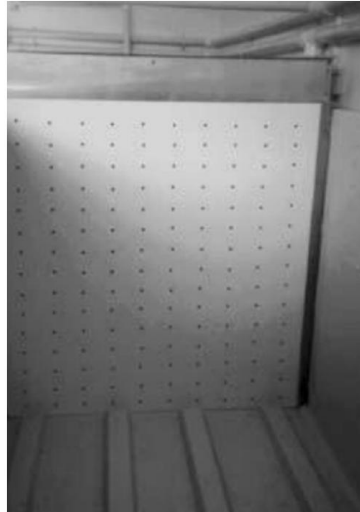
Slika 4. Perforirana pregrada ( www.seafish.org/media/Publications/SR720_Medium-scale-system.pdf )
