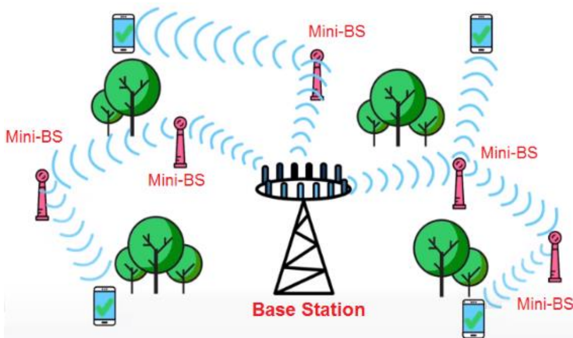
Slika 12 - Prikaz rada tehnologije malih ćelija, preuzeto sa URL: https://www.rfwireless-world.com/Terminology/5G-Small-Cells-Basics-and-Types.html
