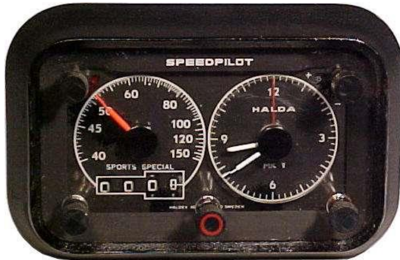
Slika 6 - Halda Speedpilot (izvor: http://www.mgaguru.com/mgtech/competition/comp203.htm )
