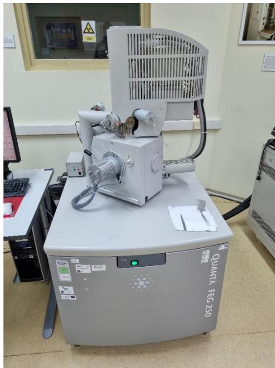
Slika 42: FEI Quanta 250 FEG SEM instrument
