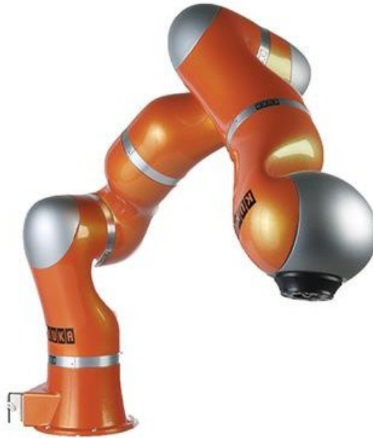
Slika 10. KUKA-in Light-Weight robot (LWR) (izvor: https://www.coboticsworld.com/portfolio-items/kuka-lwr/ )
