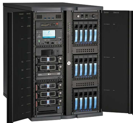
Slika 16: FRED - Forensic Recovery of Evidence Device
