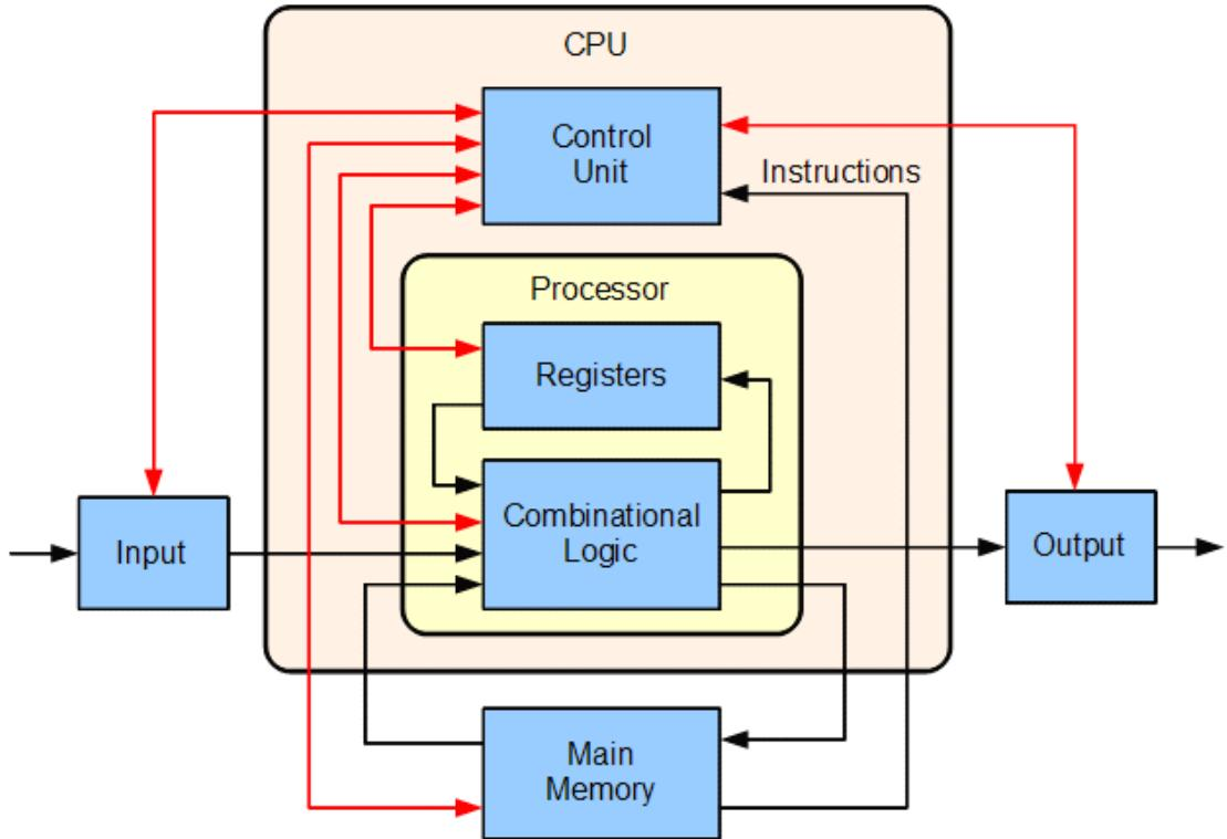
Slika 5. Blok osnovnog jednoprocorskog CPU-a (Izvor: <https://medium.com/computer-architecture-club/all-about-cpu-architecture-registers-that-you-need-to-know-31c54a892a85>)
