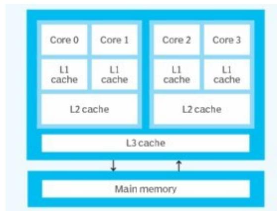
Slika 4. Arhitektura četverojezgrenog CPU-a (Izvor: [https://cdn.ttgtmedia.com/rms/onlineimages/architecture\\_of\\_quad\\_core\\_processors-h\\_half\\_column\\_mobile.png](https://cdn.ttgtmedia.com/rms/onlineimages/architecture_of_quad_core_processors-h_half_column_mobile.png))
