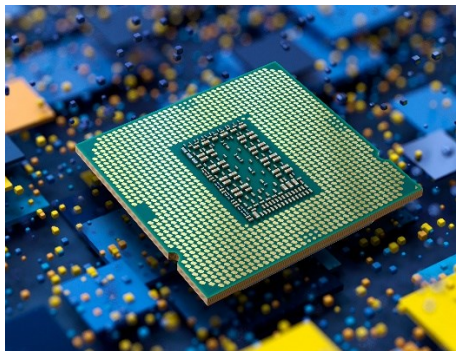
Slika 1. Prikaz CPU-a s donje strane (Izvor: https://www.trustedreviews.com/wp-content/uploads/sites/54/2021/03/Intel-Rocker-Lake-2-e1615908186584-920x614.jpg )
