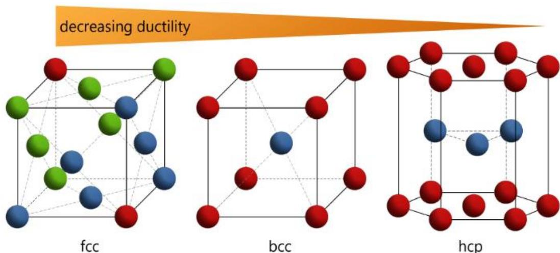
Slika 4 Tri osnovne vrste kristalnih rešetki; izvor: <https://www.tec-science.com/material-science/structure-of-metals/important-types-of-lattice-structures/>
