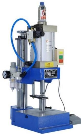
Slika 14 Pneumatska / zračna preša; izvor: [https://www.alibaba.com/product-detail/F-80-Pneumatic-Press-Machine-300KG\\_60374382031.html](https://www.alibaba.com/product-detail/F-80-Pneumatic-Press-Machine-300KG_60374382031.html)
