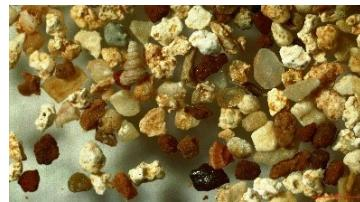
Slika 14-355 µm-H<sub>2</sub>O<sub>2</sub>
