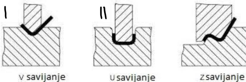
Slika 4. Primjeri savijanja u kalupima - Izvor: ("Sheet metal bending: Everything you should know explained", Shane Zang, [www.machinemfg.com](http://www.machinemfg.com), 2023.)
