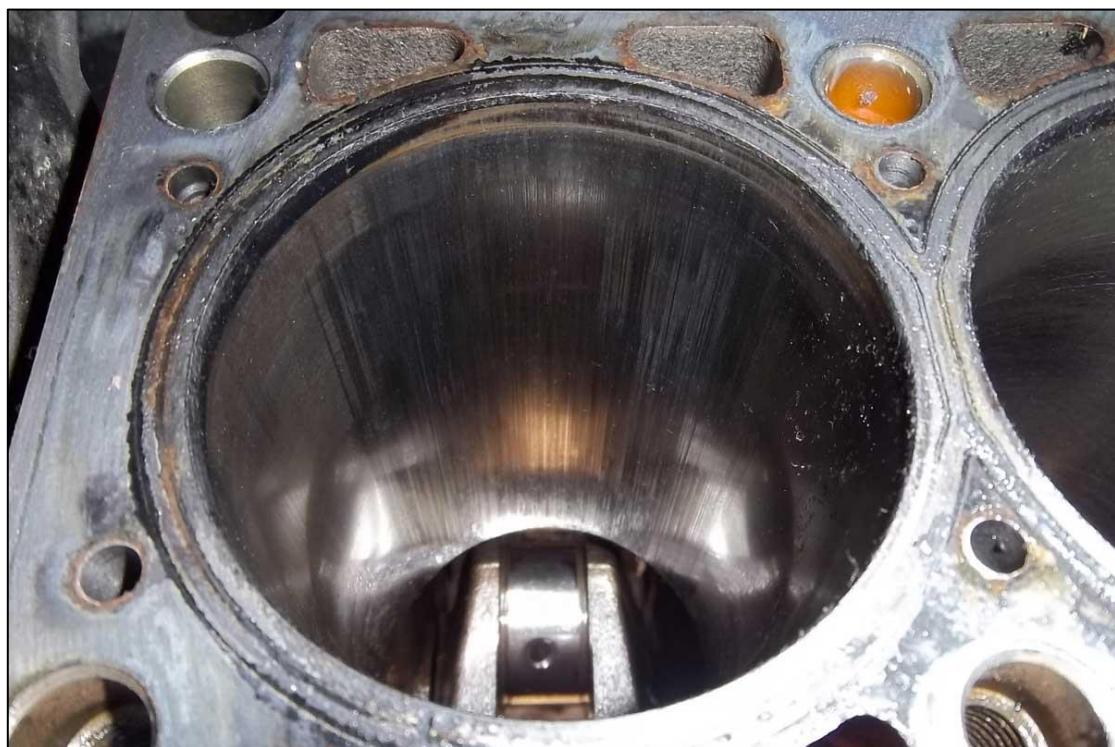
Izvor: Aurora Generators, Diesel Engine – Glazing and Carbon Buildup, 2020, dostupno na: <https://www.auroragenerators.com/post/diesel-engine-glazing-carbon-buildup>
