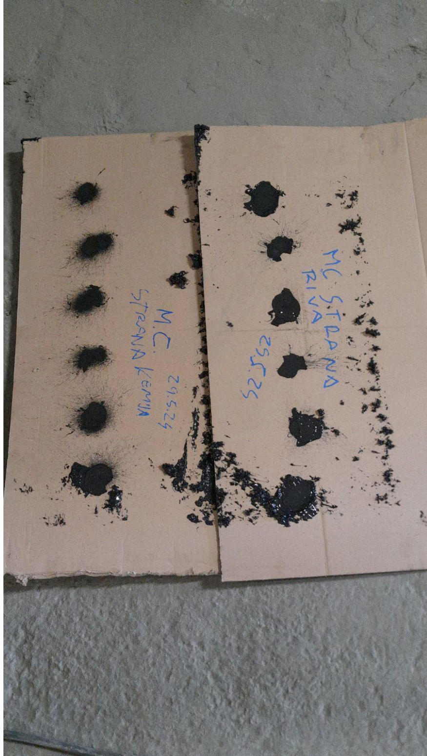
Slika 4.5.2. Spray test mlina cementa [9]
