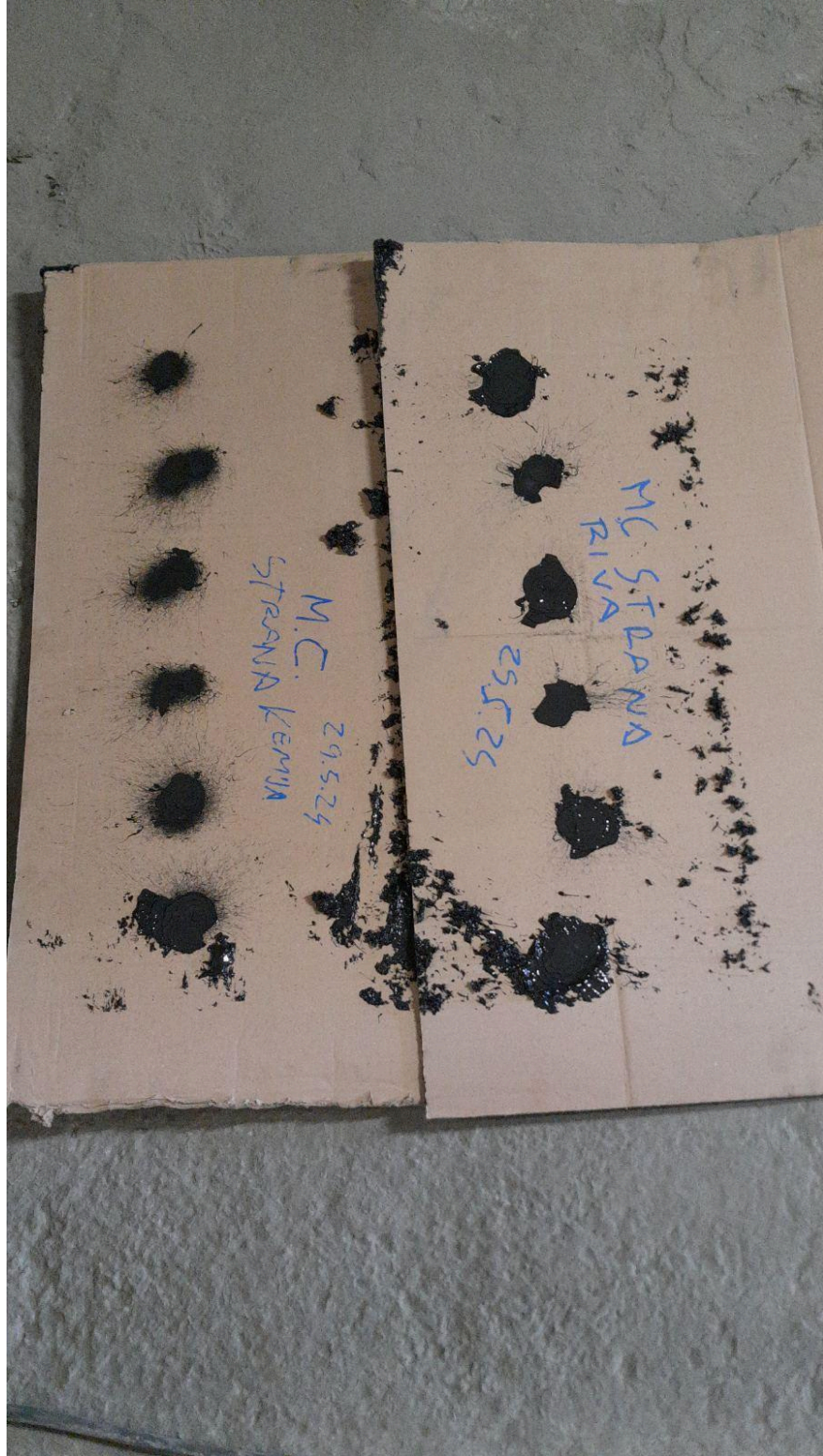
Slika 4.5.2. Spray test mlina cementa [9]
