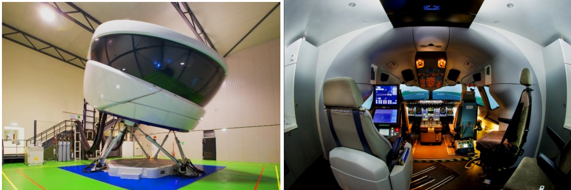
Slika 2 i 3: Sukhoi SuperJet fullflight simulator (Preuzeto od SuperJet International, 2013)
