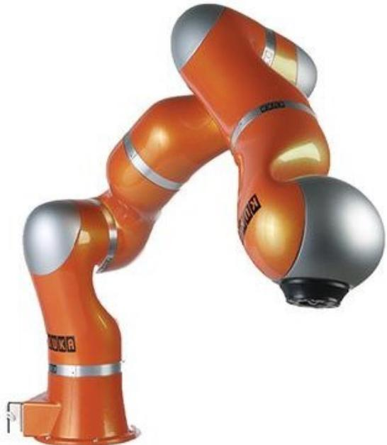
Slika 10. KUKA-in Light-Weight robot (LWR) (izvor: <https://www.coboticsworld.com/portfolio-items/kuka-lwr/>)
