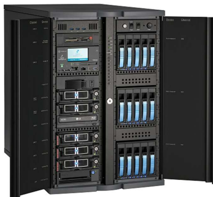
Slika 16: FRED - Forensic Recovery of Evidence Device
