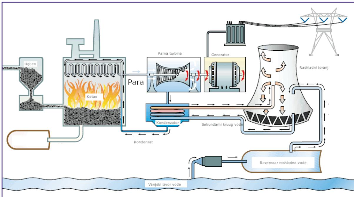
Slika 22 Pojednostavljeni dijagram radnih komponenti termoelektrane na ugljen. Izvor: Obrada autora prema [https://prd-wret.s3.us-west-2.amazonaws.com/assets/palladium/production/s3fs-public/styles/full\\_width/public-thumbnails/image/wss-wuse-thermoelectric-diagram.gif](https://prd-wret.s3.us-west-2.amazonaws.com/assets/palladium/production/s3fs-public/styles/full_width/public-thumbnails/image/wss-wuse-thermoelectric-diagram.gif)
