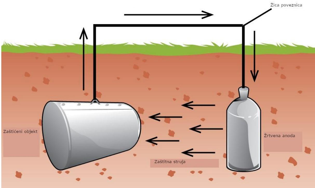
Slika 17 Dijagramske prikaze sustava pasivne katodne zaštite. Izvor: Obrada autora prema [https://cnx.org/resources/3e29d27f736f3026912fbf06dc50ded3995916d4/CNX\\_Chem\\_17\\_06\\_Protect.jpg](https://cnx.org/resources/3e29d27f736f3026912fbf06dc50ded3995916d4/CNX_Chem_17_06_Protect.jpg)
