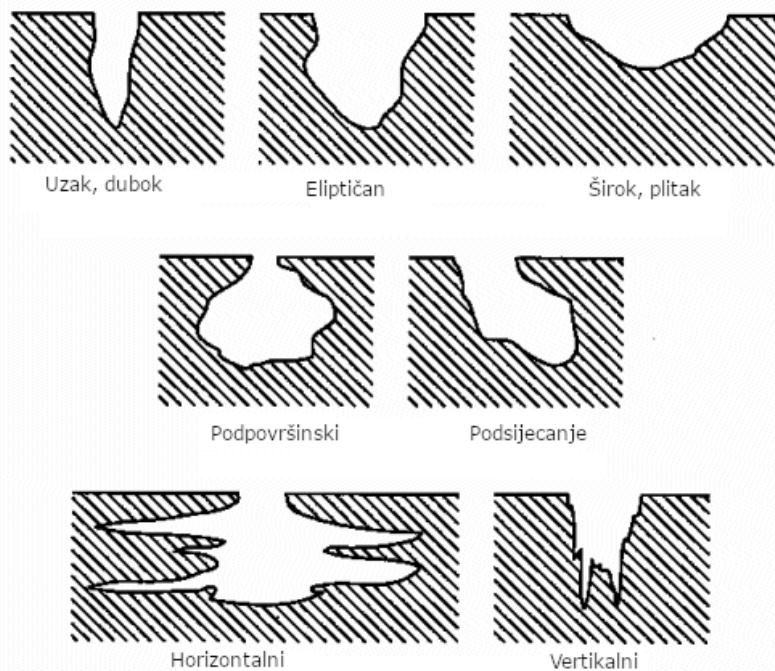
Slika 7 Poprečni presjeci različitih vrsta pitting korozije. Izvor: Obrada autora prema [https://www.corrosionclinic.com/types\\_of\\_corrosion/pitting\\_shape.gif](https://www.corrosionclinic.com/types_of_corrosion/pitting_shape.gif)
