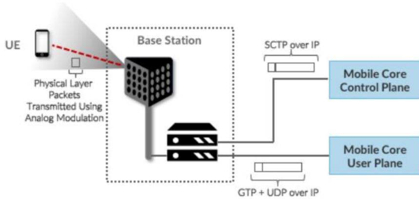
**Slika 8** Bazna stanica prema mobilnoj jezgri kontrolnog plana tunelirana preko SCTP / IP i korisnički plan tuneliran preko GTP / UDP / IP (izvor: [https://5g.systemsapproach.org/\\_images/Slide06.png](https://5g.systemsapproach.org/_images/Slide06.png))
