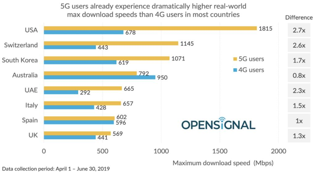
*Slika 7 - Usporedba brzina 4G i 5G mreža u više svjetskih zemalja 2019. godine, preuzeto sa URL: <https://www.opensignal.com/2019/07/08/5g-boasts-the-maximum-real-world-download-speed-by-up-to-27-times-4g-users-top-speeds>*
