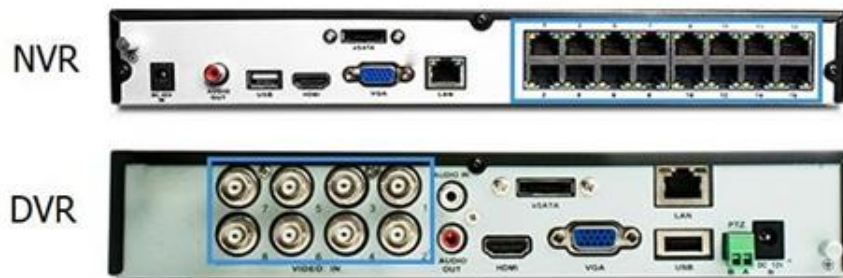
Slika 23. NVR I DVR snimači (izvor: https://getsafeandsound.com/2018/12/nvr-dvr-channels )
