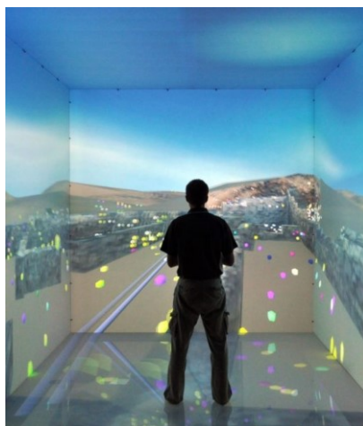
Slika 3. CAVE (Cave Automatic Virtual Environment), Izvor: mechdyne.com. (2020)
