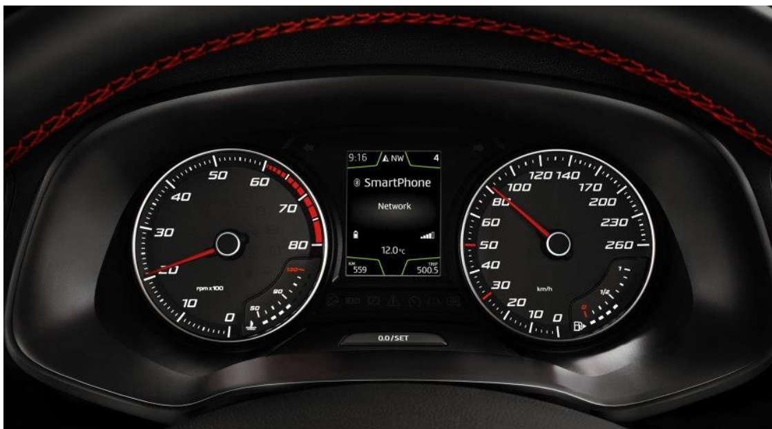
Slika 1 - putno računalo u automobilu (izvor: https://www.seat.co.uk/car-terms/o/on-board-computer.html )
