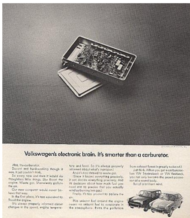
Slika 4 - Volkswagenovo prvo automobilsko računalo (1968.) (izvor: https://www.powerelectronicsnews.com/automotive-electronics-what-are-they-and-how-do-they-differ-from-normal-electronics/ )
