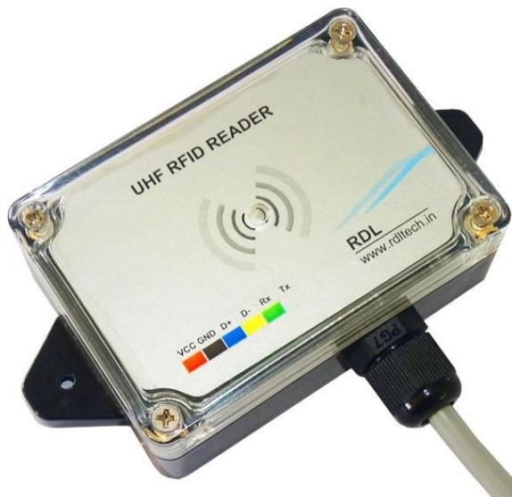
Slika 7 - Ultravisokofrekventni RFID čitač (Izvor: <https://researchdesignlab.com/uhf-rfid-reader-894.html>)
