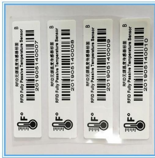
Slika 4 - RFID oznake osjetljiva na temperaturu (Izvor: [https://www.dorfidtag.com/RFID-tag-temperature-sensor-NFC-temperature-data-logger\\_2478.html](https://www.dorfidtag.com/RFID-tag-temperature-sensor-NFC-temperature-data-logger_2478.html))
