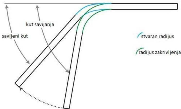
Slika 2. Povratna deformacija nakon djelovanja sile - Izvor: („Bending basics: The hows and whys of springback and springforward”, Steve Benson, [www.thefabricator.com](http://www.thefabricator.com), 2014.)
