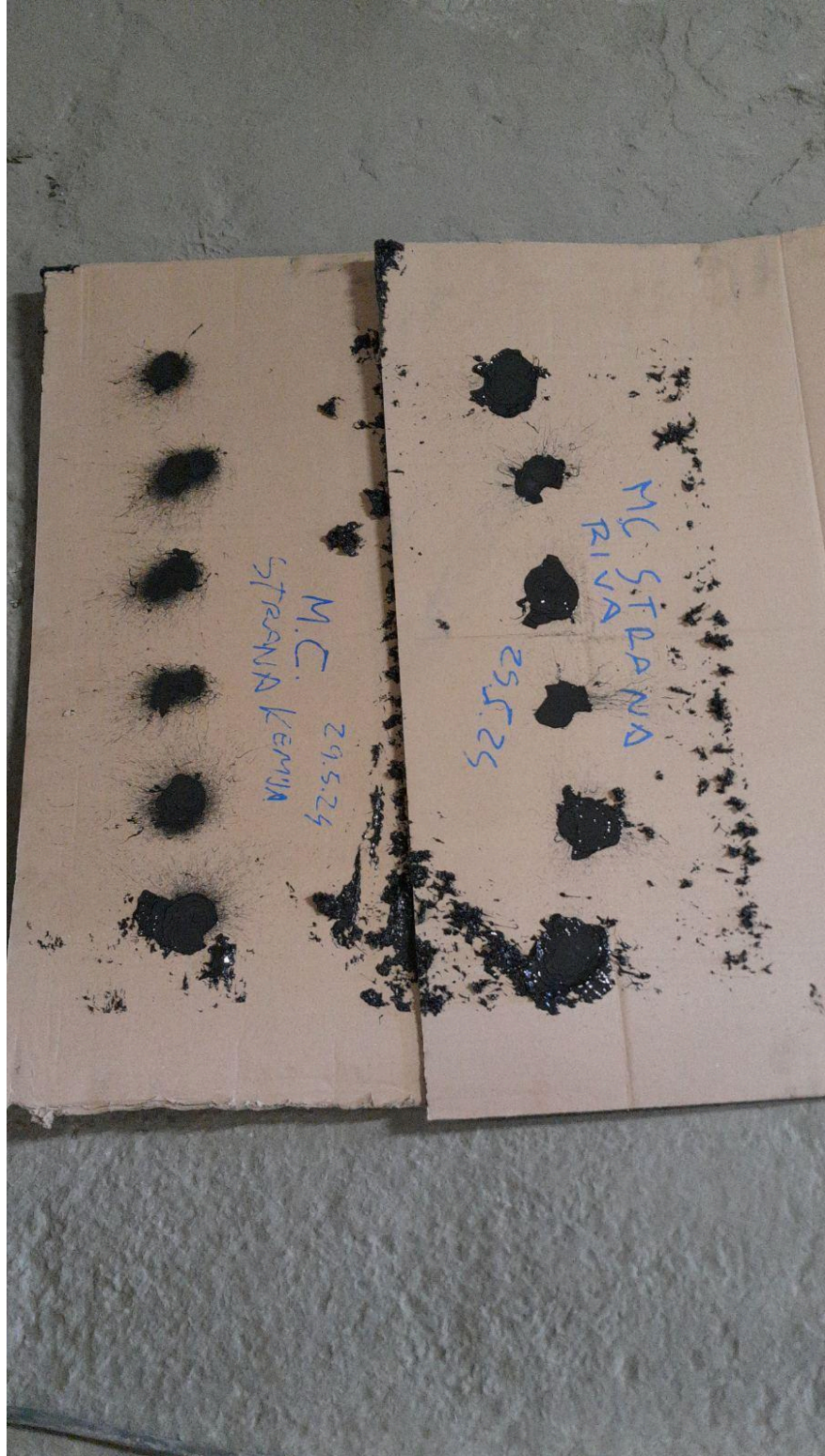
Slika 4.5.2. Spray test mlina cementa [9]
