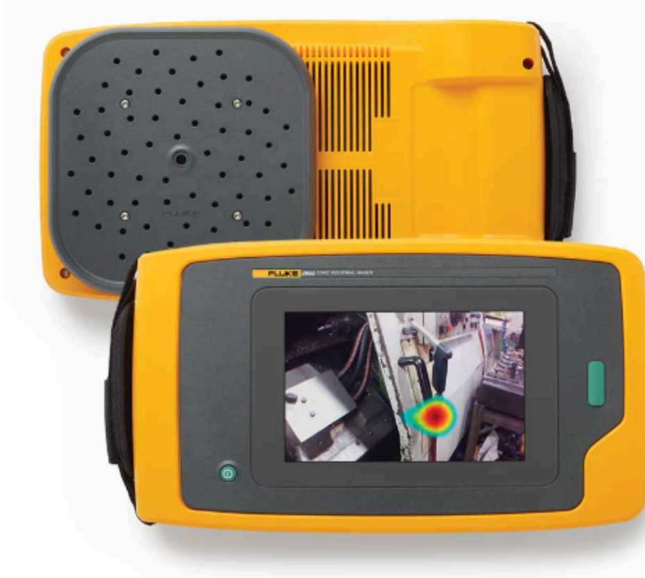
Slika 4.4.6. Fluke ii900 Industrial Acoustic Imager [13]
